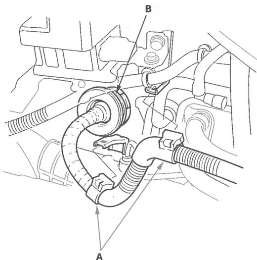
17. Remove the throttle cable (A) and cruise control cable (B) by loosening the locknuts (C), then slipping the cable ends out of the accelerator linkage. Take care not to bend the cables when removing them. Always replace any kinked cable with a new one.
