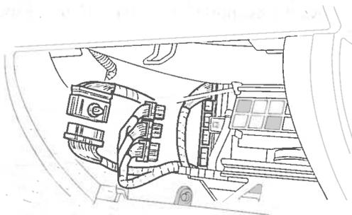
16. Remove the harness clamps (A) and grommet (B), then pull the engine wire harness through the bulkhead.
